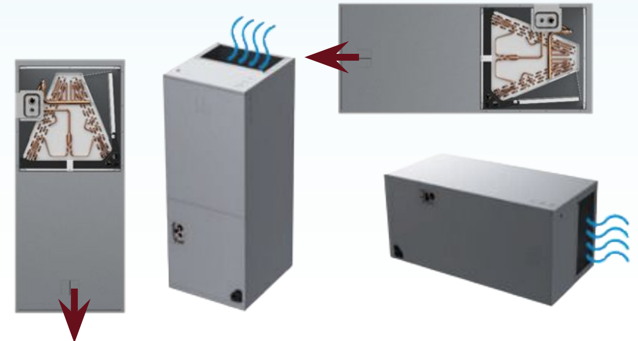
A vertical up flow unit may be converted to vertical down flow, by removing the panel and indoor coil and reinstall 180° from original position. Same for horizontal left flow.
